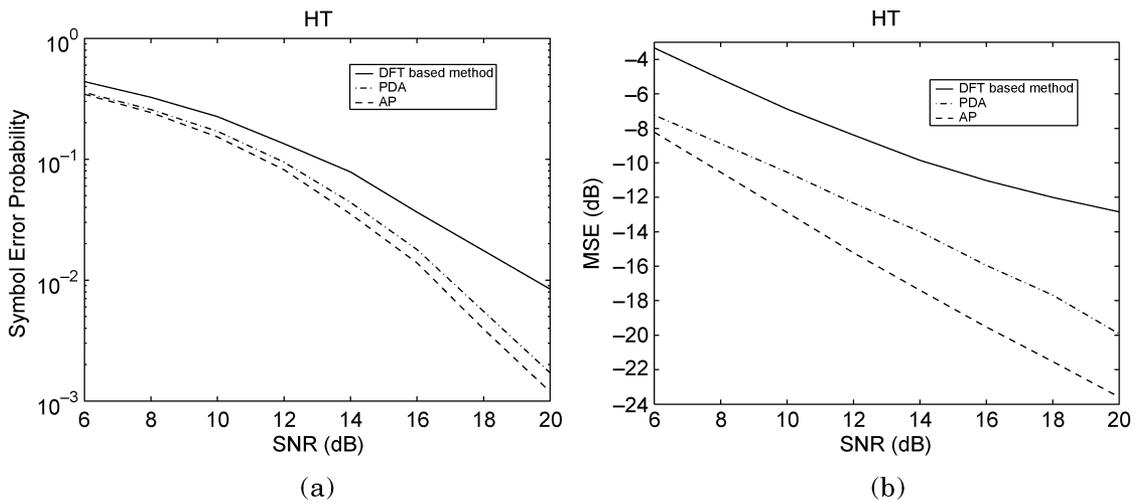
Fig. 3. Performance comparisons of different channel estimators for the HT channel with 40-Hz Doppler frequency. (a) Symbol error probability. (b) MSE.
