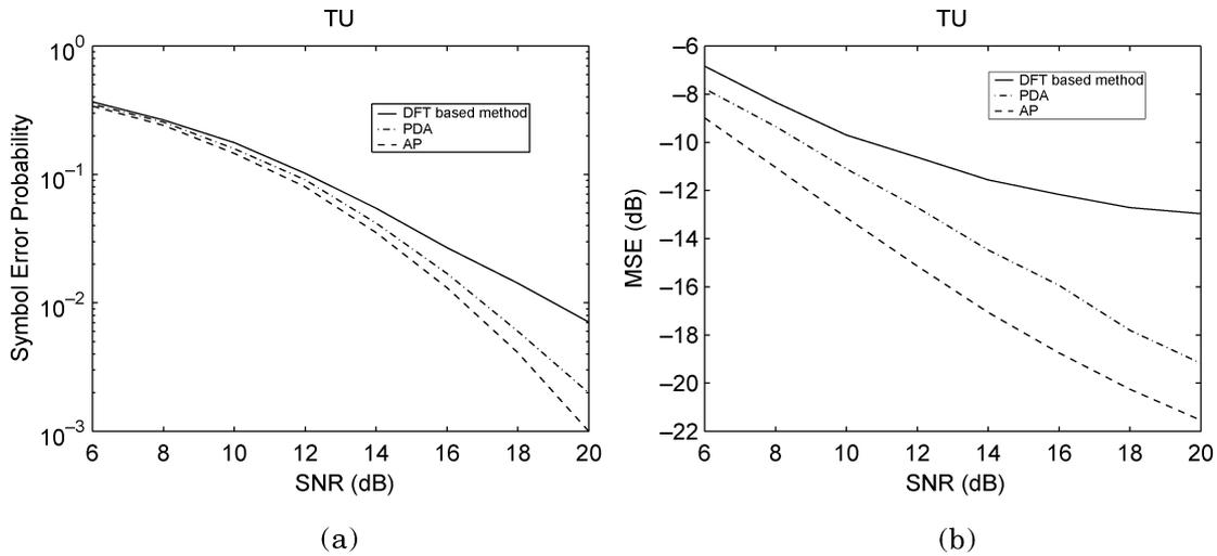
Fig. 2. Performance comparisons of different channel estimators for the TU channel with 40 Hz Doppler frequency. (a) Symbol error probability. (b) MSE.
