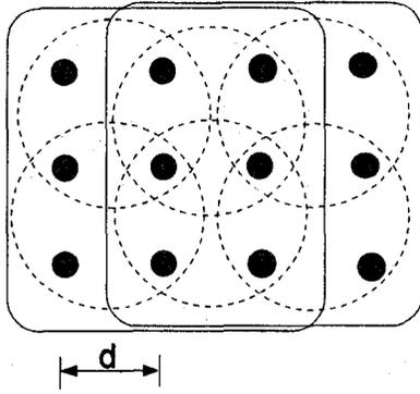
Fig. 9. Twelve-sensor rectangle array with spacing  $d$ .
