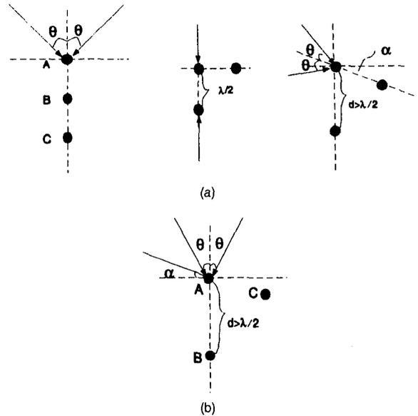
Fig. 2. Three-sensor array structures that can cause ambiguities.
