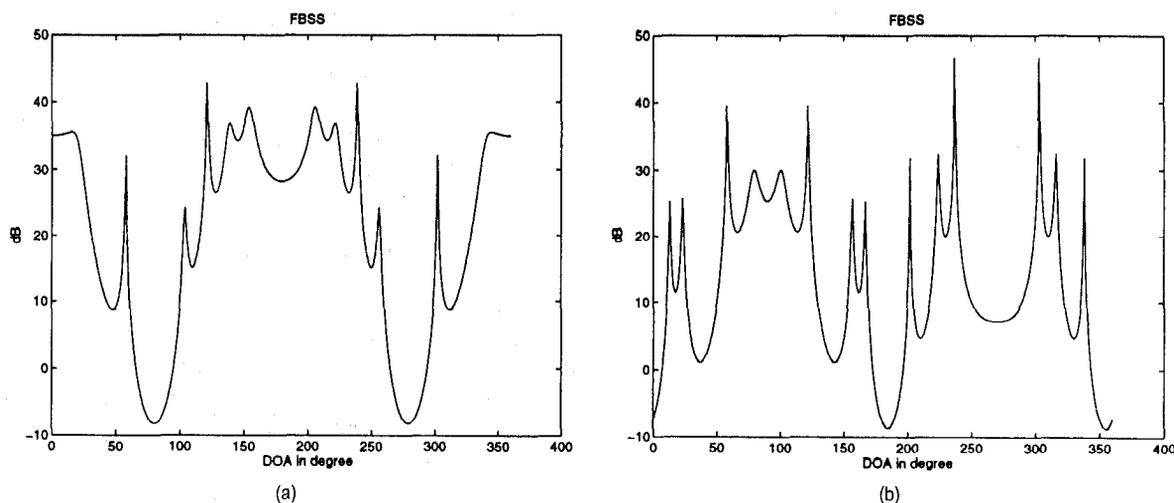
Fig. 6. DOA estimation of four groups of coherent signals at  $(10^\circ, 20^\circ, 100^\circ)$ ,  $(120^\circ)$ ,  $(200^\circ, 220^\circ)$ ,  $(300^\circ)$  based on two crossed linear arrays. (a) Horizontally positioned linear array. (b) Vertically positioned linear array.
