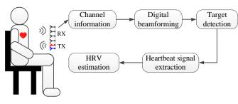
Fig. 1: Processing flow of mmHRV.
