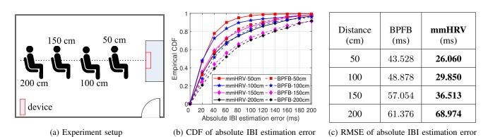
Fig. 10: Experiment setup and the absolute IBI estimation results versus distance.
