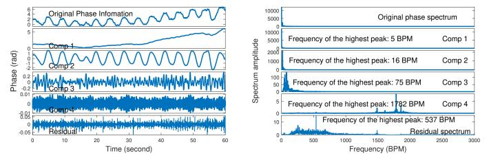
(a) Decomposition of a typical phase signal in time domain
