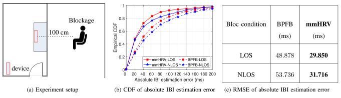
Fig. 13: Experiment setup and the absolute IBI estimation results versus blockage.
