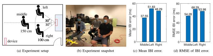
Fig. 15: Mean and RMSE of the absolute IBI estimation error of multiple users.
