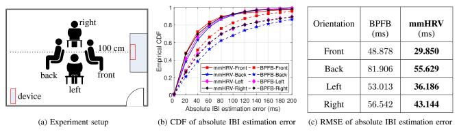
Fig. 11: Experiment setup and the absolute IBI estimation results versus orientation.
