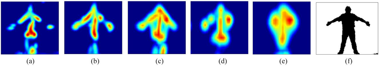
Fig. 11. Impact of distance on human imaging. A subject stands in front of the device with varying distances and performs the same posture, as illustrated in the Kinect depth image. (a) 1m. (b) 1.5m. (c) 2m. (d) 2.5m. (e) 3m. (f) Kinect.
