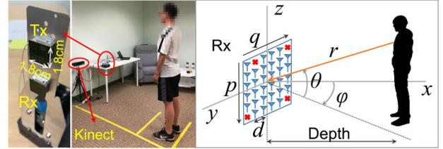
Fig. 2. Device setup and coordinate system.  $\theta$  and  $\phi$  denote the elevation and azimuth, respectively, and  $r$  denotes the range from the device to the reflector. The antenna array contains 32 elements in a  $6 \times 6$  layout, with four missing locations marked by red crosses.
