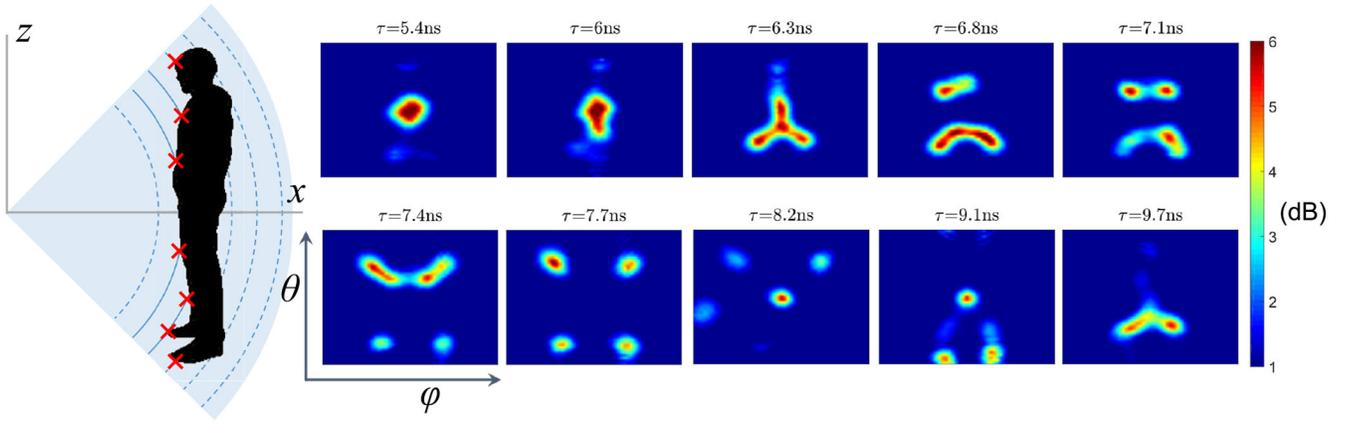
Fig. 3. Spatial spectrum for different propagation delay  $\tau$ , which demonstrate the sparsity of the reflected signals off the target at individual range/delay.
