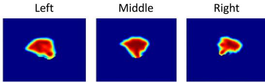
Fig. 19. Imaging for a human face. A person sits 30 cm away from the device and faces the device. Left: The person tilts the head to the left; Middle: The person keeps the head straight; Right: The person tilts the head to the right.
