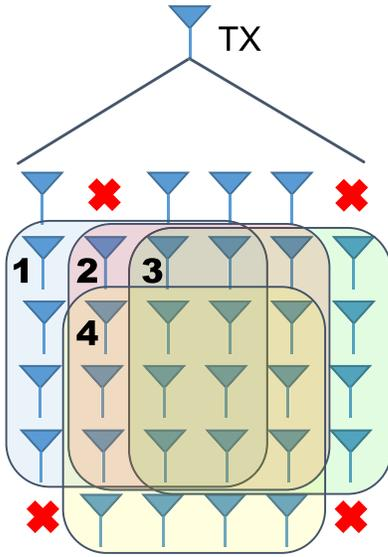
Fig. 4. SS. Four  $4 \times 4$  subarrays are established from the  $6 \times 6$  receive array.
