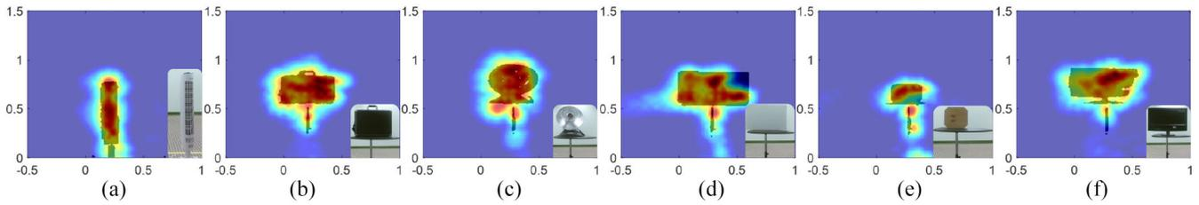
Fig. 15. Imaging for different static objects. Objects with different shapes, sizes, materials, and surface conditions are tested. The objects are placed about 1.5 m away from the device. The shadow overlays show the ground truths obtained by Kinect. (a) Fan. (b) Plastic suitcase. (c) Heater. (d) Large wood panel. (e) Small wood panel. (f) Monitor.
