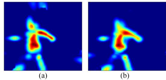
Fig. 14. Imaging on (a) Tx/ (b) Rx array. The quality of the image obtained on Rx array is better than that obtained on the Tx array.
