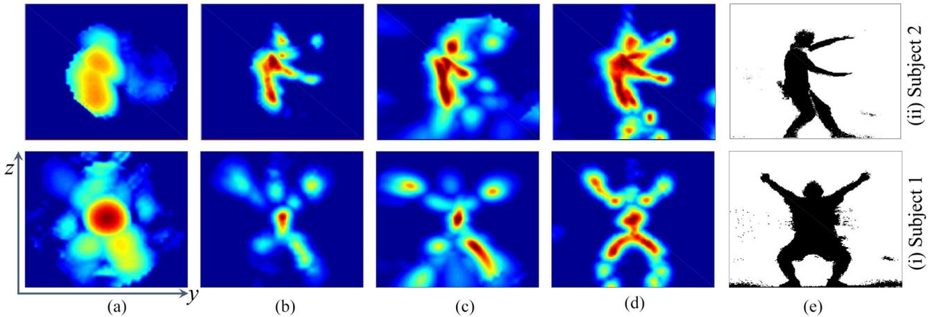
Fig. 9. Examples of the imaging results. (a)–(d) show the examples of the obtained images by different spatial spectrum estimators. The color indicates the value of  $P_i^*$  for the  $i$ th detected point, and the higher value, the redder color (c) and (d) are the results by mmEye with SS and JTS, respectively (e) is obtained as the ground truth by a Kinect depth sensor.
