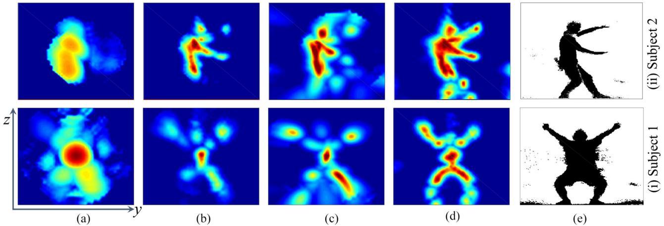
Fig. 9. Examples of the imaging results. (a)–(d) show the examples of the obtained images by different spatial spectrum estimators. The color indicates the value of  $P_i^*$  for the  $i$ th detected point, and the higher value, the redder color (c) and (d) are the results by mmEye with SS and JTS, respectively (e) is obtained as the ground truth by a Kinect depth sensor.
