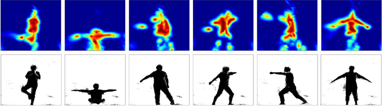
Fig. 1. Example imaging results produced by mmEye (top) compared with Kinect (bottom). The subjects are about 1 m away from the device.
