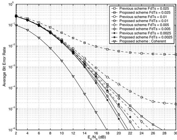
Fig. 4: Two-ray power delay profile,  $M_t = 3$ ,  $M_r = 1$ , and  $R \approx 1$  b/s/Hz.
