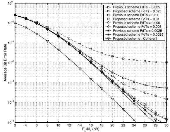
Fig. 3: TU power delay profile,  $M_t = 2$ ,  $M_r = 1$ , and  $R = 1 \text{ b/s/Hz}$ .
