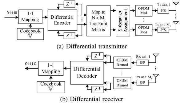
Fig. 1: Description of the differential MIMO-OFDM system.
