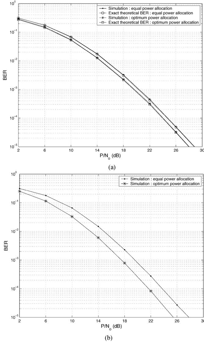
Fig. 4. DiffAF scheme with DQPSK: two relays, optimum power allocation strategy. (a)  $\sigma_{s,d}^2 = 1$ ,  $\sigma_{s,r_i}^2 = 10$ , and  $\sigma_{r_i,d}^2 = 1$ . (b)  $\sigma_{s,d}^2 = \sigma_{s,r_i}^2 = 1$  and  $\sigma_{r_i,d}^2 = 10$ .
