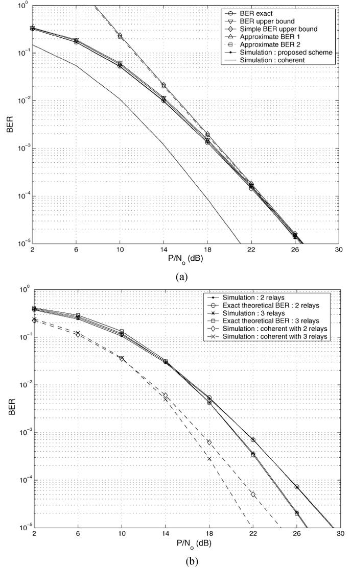
Fig. 3. DiffAF scheme with equal power allocation strategy and  $\sigma_{s,d}^2 = \sigma_{s,r_i}^2 = \sigma_{r_i,d}^2 = 1$ . (a) DBPSK: two relays. (b) DQPSK: two and three relays.
