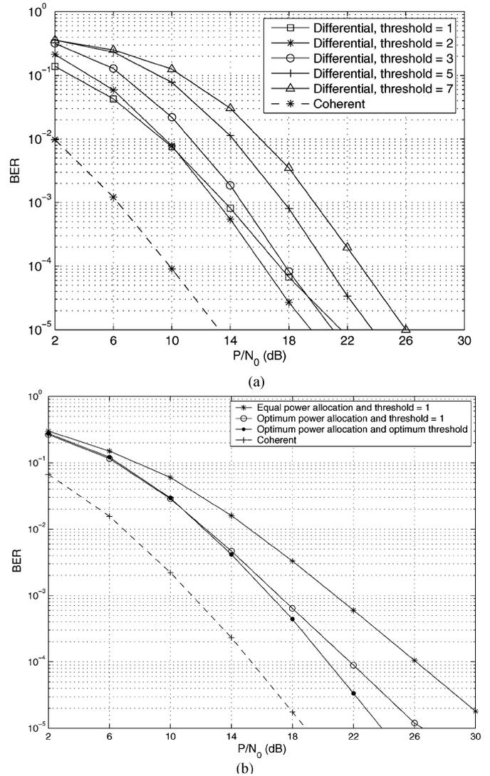
Fig. 7. DiffDF scheme with  $\sigma_{s,d}^2 = \sigma_{s,r_i}^2 = 1$ ,  $\sigma_{r_i,d}^2 = 10$ . (a) DBPSK: three relays, fixed power allocation, but different thresholds. (b) DQPSK: two relays, different power allocation and thresholds.
