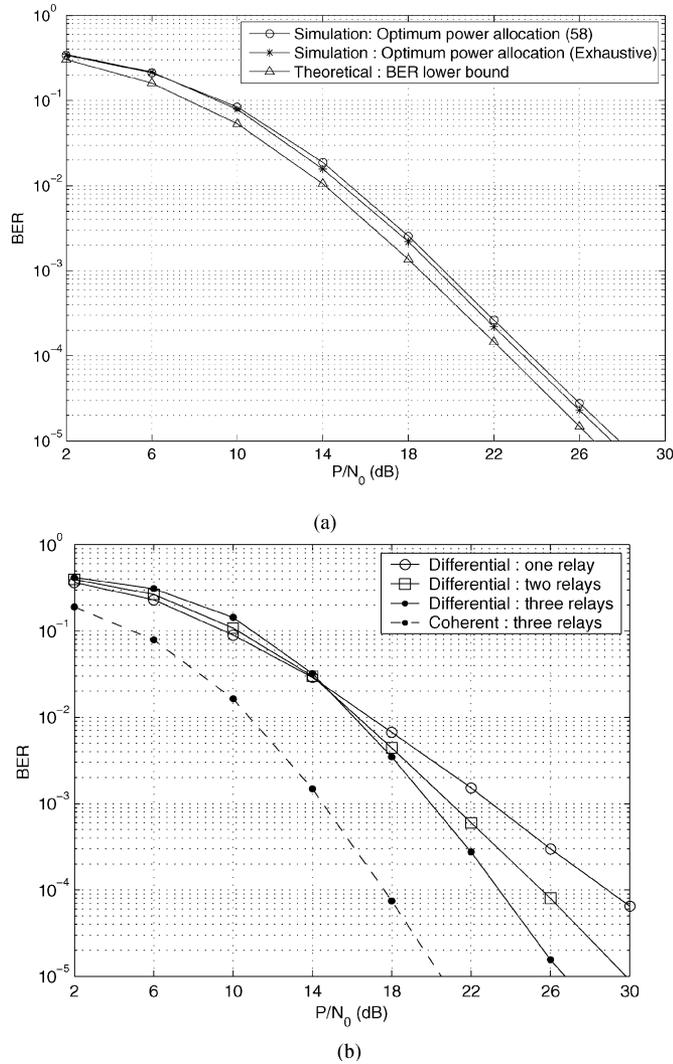
Fig. 6. DiffDF with DQPSK. (a) Optimum power allocation (58) and exhaustive optimum power allocation  $\sigma_{s,d}^2 = \sigma_{s,r_1}^2 = \sigma_{r_i,d}^2 = 1$  and  $\sigma_{s,r_2}^2 = 5$ . (b) Different number of relays  $\sigma_{s,d}^2 = \sigma_{s,r_i}^2 = \sigma_{r_i,d}^2 = 1$ .
