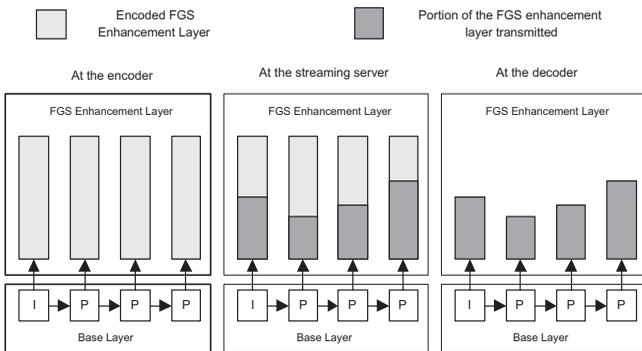
Fig. 2. Streaming video using MPEG-4 FGS.
