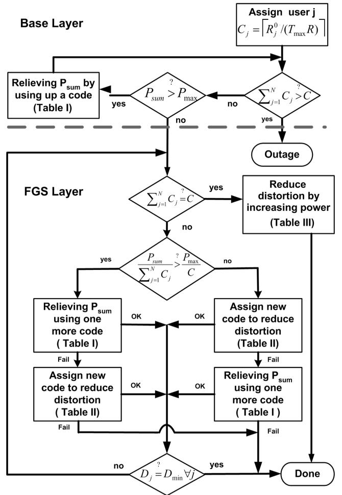
Fig. 3. Distortion Management Algorithm for base layer and FGS layer.
