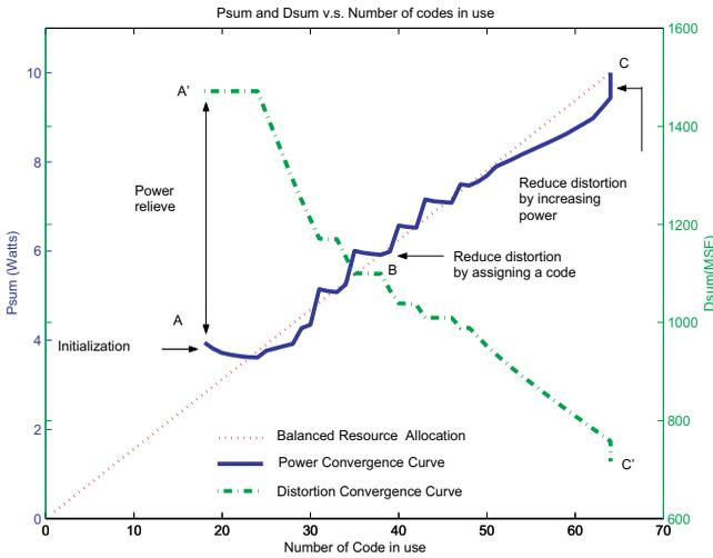
Fig. 4. Power and distortion vs. the number of assigned codes.
