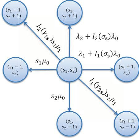
Fig. 2. State transition diagram of the wireless access network association system.
