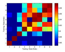
Fig. 10. Resonance strength map with RX on LOC B and TX on the first green dot (axis 1).
