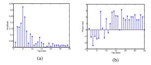
Fig. 4. Example of indoor CSI. (a) Amplitude of CSI. (b) Phase of CSI.
