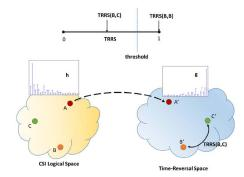
Fig. 3. Mapping between the CSI logical space and the TR space.
