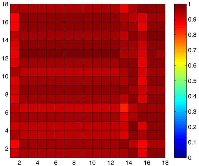
Fig. 7. TR resonating strength between CIRs of the forward link and those of the backward link.
