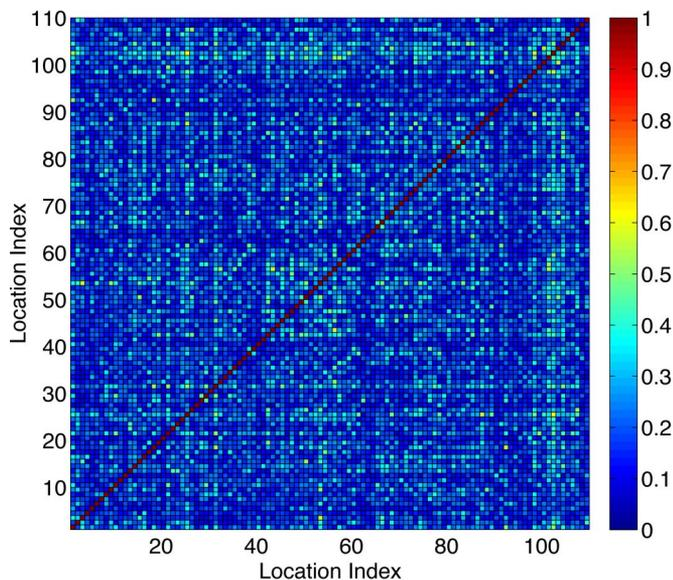
Fig. 12. Focusing gain  $\eta^2$  of all grid points by moving the intended location within 1 m by 0.9 m area. Every dot in the figure stands for one grid point where two neighboring grids points are 10 cm away from each other. The horizontal/vertical axis is the location index with 1-D representation. Each value in  $(i, j)$  represents the focusing gain at location  $j$  (location index with 1-D representation) when the intended location is  $i$  (location index with 1-D representation).
