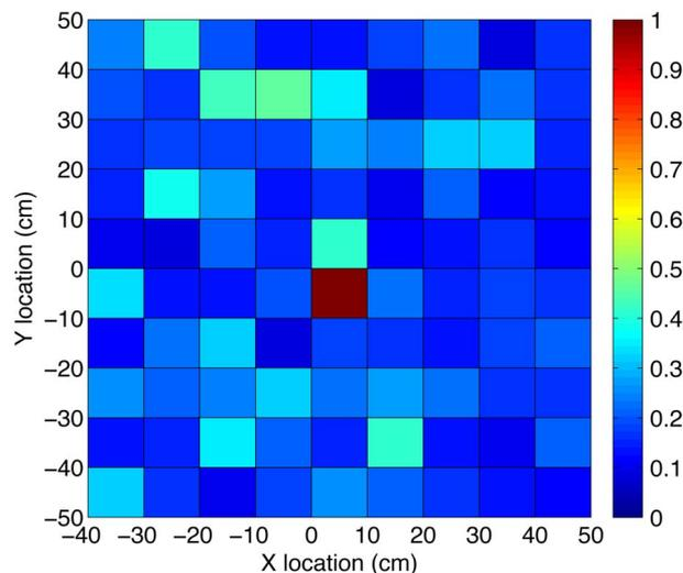
Fig. 13. Geographic distribution of  $\eta^2$  with the intended location at the center of the area of interest.
