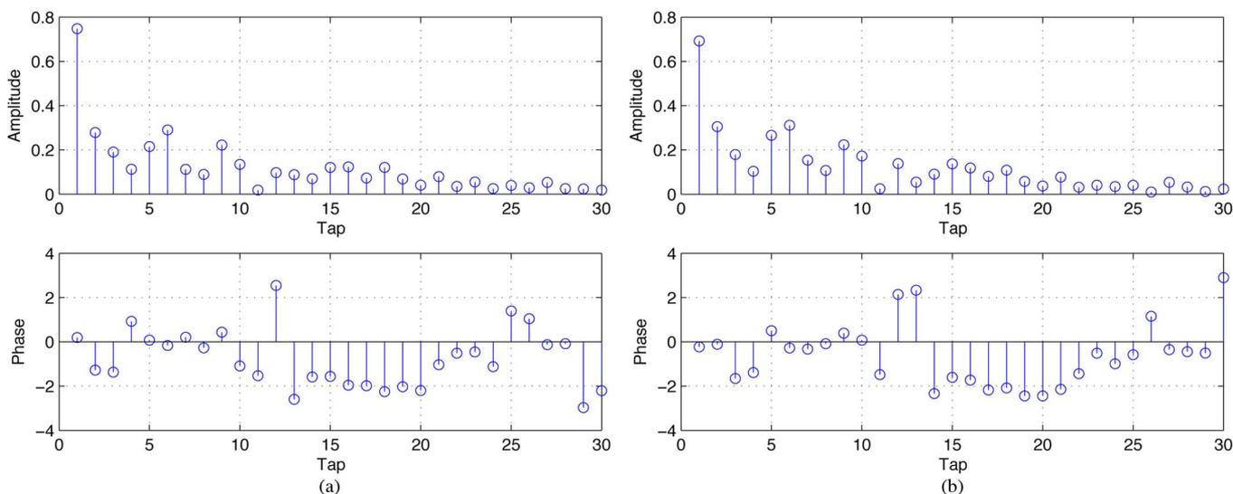
Fig. 5. Evaluation of channel reciprocity. (a) CIR of the forward link. (b) CIR of the backward link.
