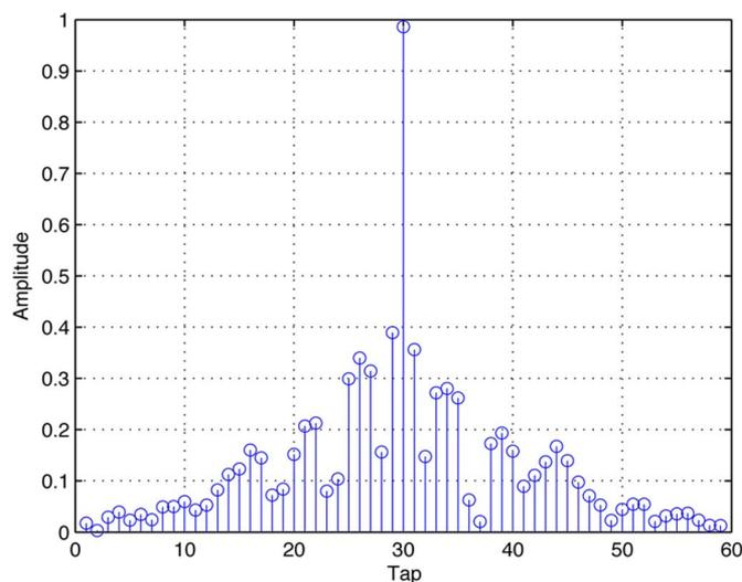
Fig. 6. Cross correlation between the CIR of the forward link and that of the backward link. Note that the center tap is the TR resonating strength between the CIR of the forward link and that of the backward link.
