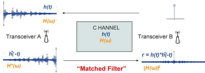
Fig. 2. TR signal processing principle.
