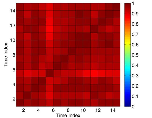
Fig. 10. Evaluation of channel stationarity under minor environment change using TR resonating strength between any two CIRs collected with a person walking around.
