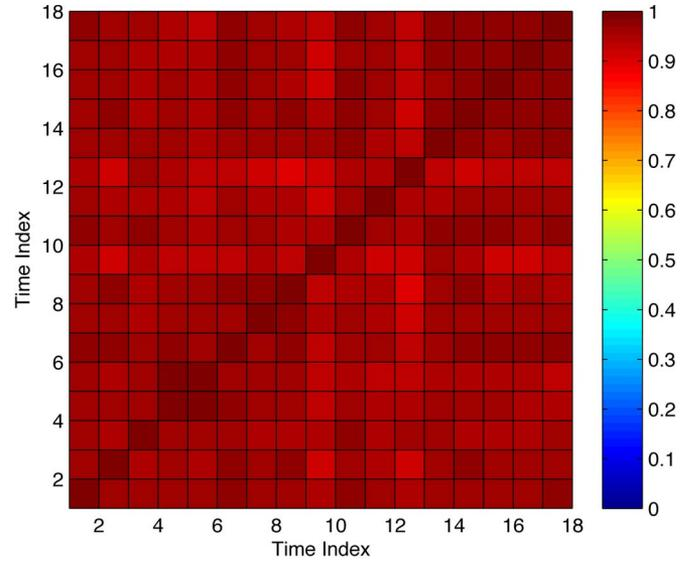
Fig. 9. Evaluation of long temporal stationarity using the TR resonating strength between any two CIRs from the 18 CIRs collected over a weekend between the AP and the TD.
