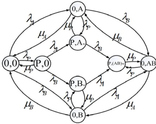
Fig. 3. The rate diagram of CTMC with queuing.
