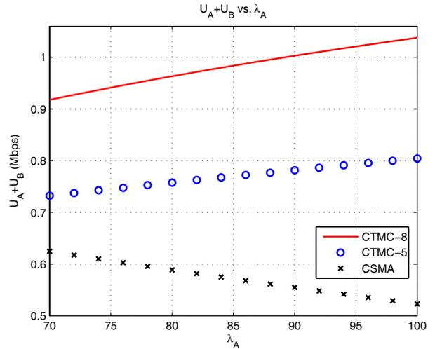
Fig. 10. Overall throughput for CTMC-5, CTMC-8 and CSMA.
