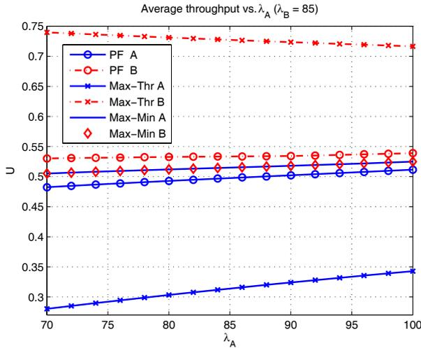
Fig. 9. Average throughput vs.  $\lambda_A$  (asymmetric-interference,  $\lambda_B = 85$   $s^{-1}$ ).
