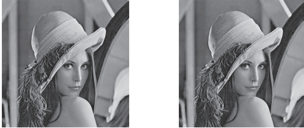
Fig. 2. Left: An image compressed using the SPIHT algorithm at a bit rate of 3 bits per pixel before the use of entropy coding. Right: The same image after anti-forensic dither has been applied to its wavelet coefficients.
