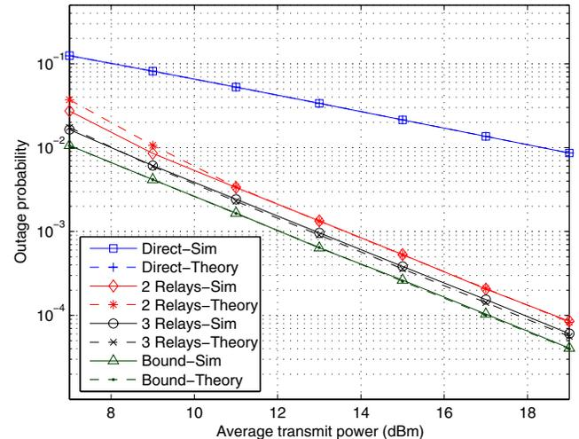
Fig. 2: Outage probability versus average transmitted power.
