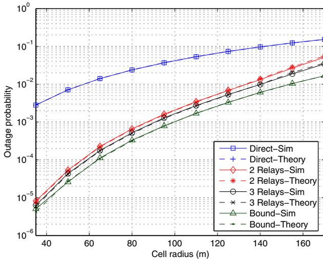
Fig. 1: Outage probability versus cell radius.
