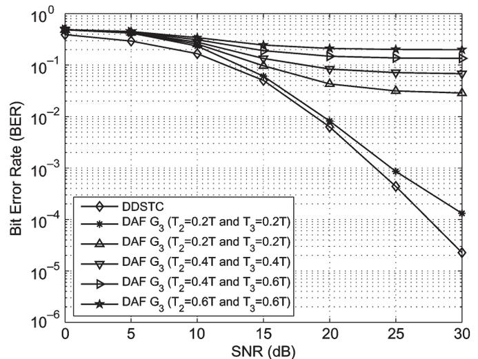
Fig. 7. BER performance with propagation delay mismatch. Three relay cases.
