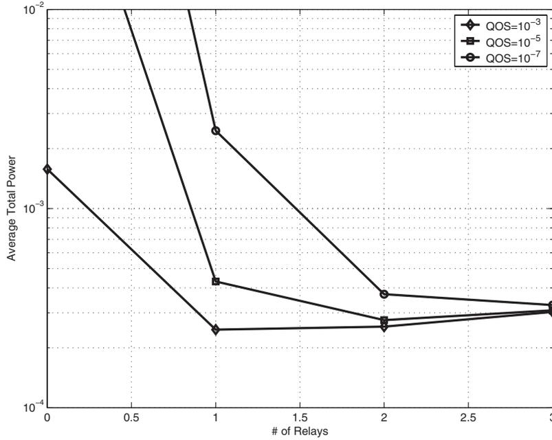
Fig. 10. Optimal consumed power versus number of relays for different values of required outage probability.
