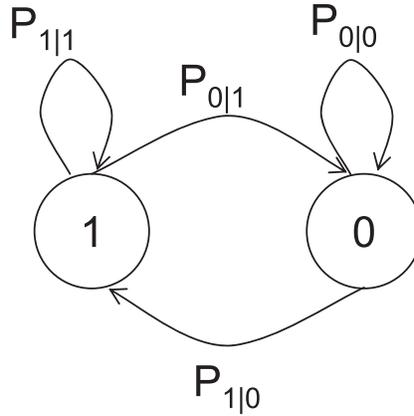
Fig. 3. Modeling the channel by a two (on-off) state Markov chain to study the time correlation.
