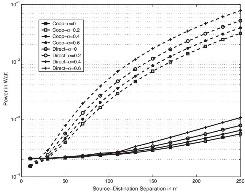
Fig. 6. Optimal power consumption for both cooperation and direct transmission scenarios for different values of power amplifier loss  $\alpha$ .
