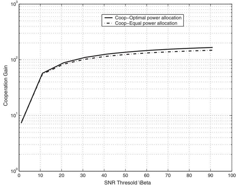
Fig. 5. Cooperation gain versus the SNR threshold  $\beta$ .
