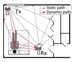
Fig. 3: Multipath propagation
