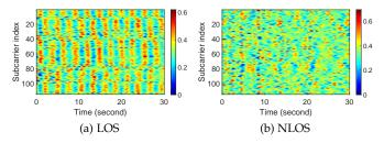
Fig. 4: The normalized CSI power response matrix with the presence of breathing signals. To facilitate the visualization, G(t,f) is smoothed and normalized to the same amplitude over time for each subcarrier.
