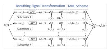
Fig. 8: The diagram of MRC on ACF of breathing signal.
