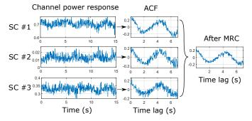
Fig. 9: Example of MRC scheme for breathing signal maximization. Subcarrier (SC) 1, 2 and 3 rank the first, sixth and tenth respectively among the 114 subcarriers from a link according to  $\hat{k}(f)$ .
