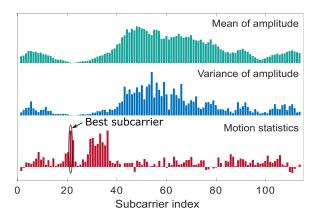
Fig. 10: Comparison of the subcarrier selection schemes. The best subcarriers selected by the mean and variance are merely ranked 113-th and 95-th, respectively, when considering their motion statistics.
