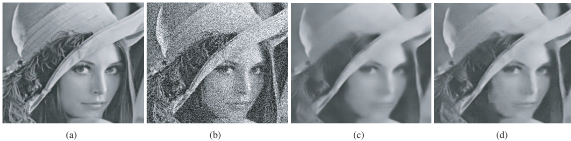
Fig. 4. The visual quality comparison for Lena with \sigma = 45 : (a) original image; (b) noisy image; (c) the result generated by the nonlocal method; (d) the result generated by the proposed approach.
