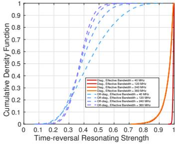
Fig. 4: CDF of the TRRS for the diagonal and off-diagonal elements.
