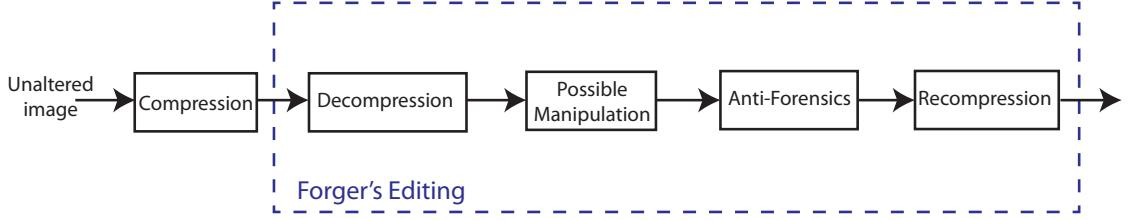
Figure 5.2: The system model considered in this chapter.
