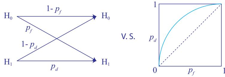
Figure 4.4: Compare a simple hypothesis channel and a ROC curve.
