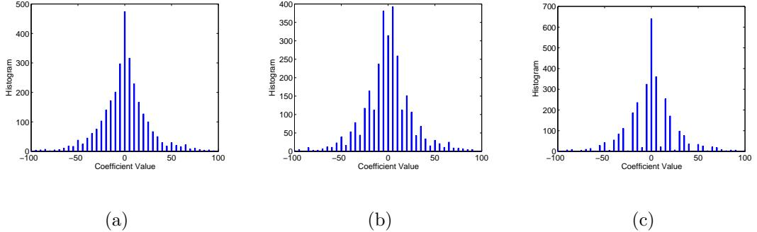
Figure 5.1: Histograms of DCT coefficients subtracted from sub-band (0,2) of a natural image been (a) single compressed with specific quantization step 5, (b) doubly compressed with quantization step 3 followed by 5, and (c) doubly compressed with quantization step 7 followed by 5.
