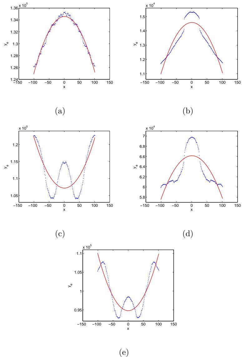
Figure 4.7: The noise energy pattern signal (dotted blue lines) extracted from the DFT of the p-map and their polynomial fitting curves (solid red lines) for (a) an unaltered image, (b) a resized image, (c) a blurred image, (d) a blurred then resized image, and (e) a resized then blurred image.
