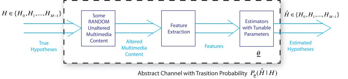
Figure 4.3: A typical process of estimating the hypotheses.
