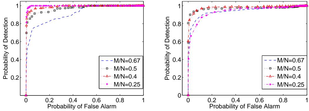
Figure 2.14: ROC curves of the first (left) and second (right) step detections on coefficients of DWT sub-band 3 under different compression ratios of compressive sensing.
