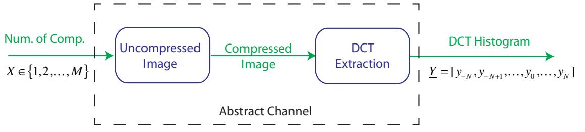
Figure 3.3: Channel model for the example of multiple compression detection forensics.
