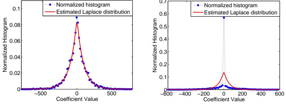
Figure 2.5: Fitting the histogram of the observed signal to the estimated signal distribution. The Laplace distribution was used to generate each sample of the nearly sparse signal. The left figure shows the fitting result when this signal was obtained by traditional sensing, while the right one shows the result for a when the signal was compressively sensed.
