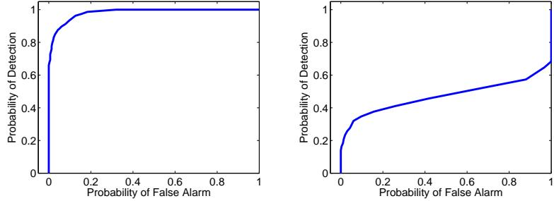
Figure 2.8: ROC curves obtained by using the proposed scheme in Section 2.3.2 to identify compressively sensed images from traditionally sensed images (left) and to identify compressively sensed images from traditionally sensed but JPEG 2000 compressed images (right).
