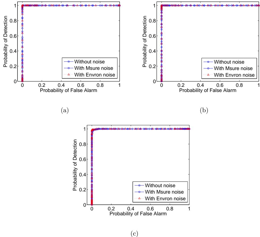
Figure 2.12: ROC curves of distribution-based detection on nearly sparse signals and nearly sparse signals in the presence of noise for (a)  $M/N=0.1$ , (b)  $M/N=0.4$  and (c)  $M/N=0.9$ . ‘Msure’ is short for measurement and ‘Envron’ is short for environment.
