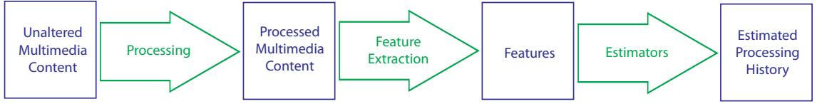
Figure 3.1: Typical process that a multimedia signal may go through when considering forensics.
