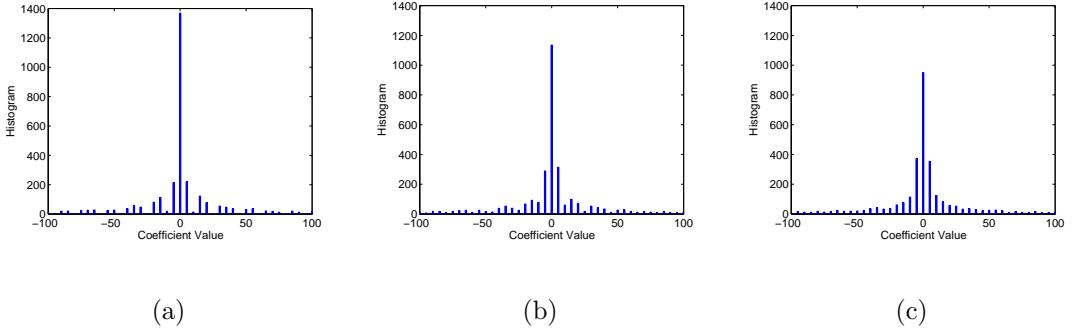
Figure 5.5: Histograms of DCT coefficients of an anti-forensically modified and double compressed image with anti-forensic strength (a)  $\alpha = 0$ , (b)  $\alpha = 0.4$ , and (c)  $\alpha = 1$ .
