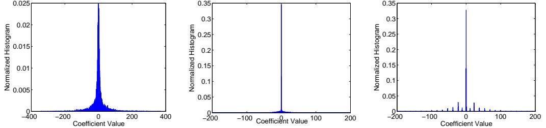
Figure 2.6: Histograms of DWT coefficients taken from uncompressed Lena (left), the same image after JPEG 2000 compression (right), and the reconstructed compressively sensed Lena (center).
