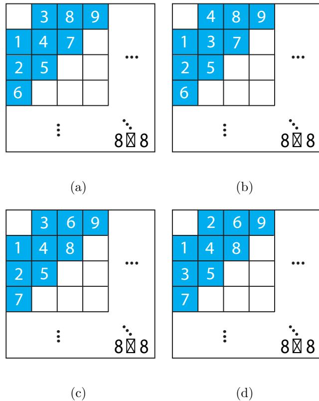
Figure 3.12: The best 9 DCT subbands (shown as blue cells) for detection, which yield the highest forensicabilities for (a)  $M = 2$ , (b)  $M = 3$ , (c)  $M = 4$  and (d)  $M = 5$ . Numbers 1 through 9 represent the order of these subbands regarding their forensicabilities from the highest to the lowest.
