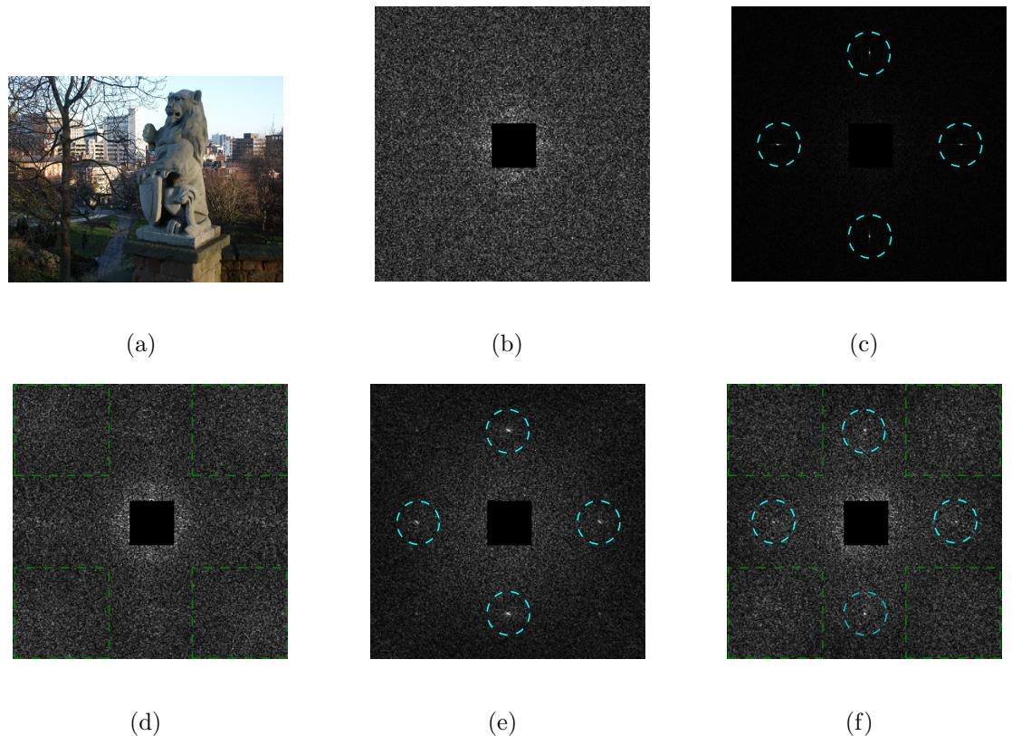
Figure 4.1: Fingerprints for detecting the order of resizing and blurring. (a) and (b) are the original image and the DFT of its p-map, respectively. (c) - (f) show the DFT of the p-map of (c) the resized image, (d) the blurred image, (e) the blurred then resized image, and (f) the resized then blurred image. Resizing factor is 1.5 (upsampling). Gaussian blur is used with variance 1. Regions of interests are highlighted by dotted squares and circles.
