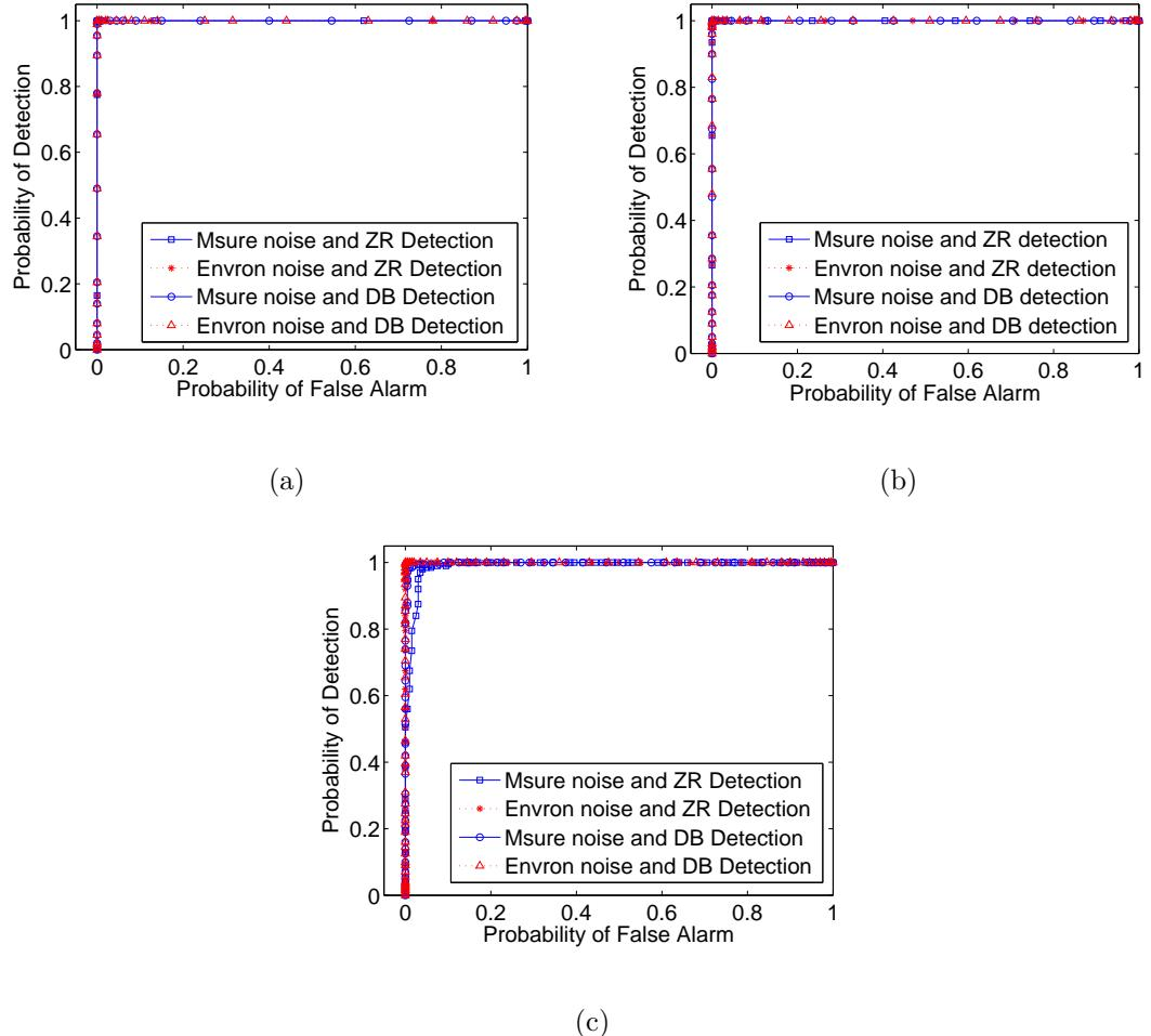
Figure 2.10: ROC curves of zero ratio detector and distribution-based detector on signals modeled as sparse signals in the presence of noise for (a)  $M/N=0.1$ , (b)  $M/N=0.4$  and (c)  $M/N=0.9$ . ‘Msure’ is short for measurement and ‘Envron’ is short for environment. ‘ZR’ denotes the zero ratio detector and ‘DB’ denotes the distribution-based detector.
