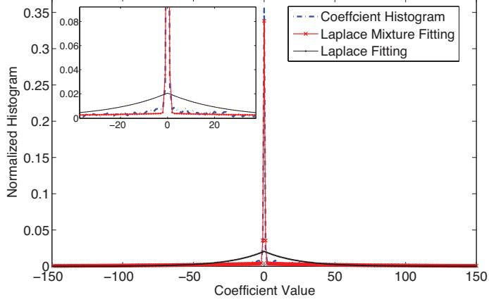
Figure 2.9: Fit the coefficient histogram of compressively sensed Lena with both Laplace model and Laplace mixture model. Coefficients are taken from the third subband after 6-level DWT decomposition with wavelet basis ‘bior4.4’.
