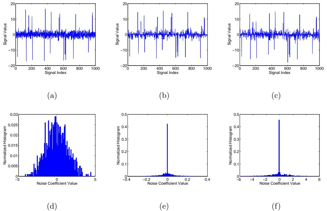
Figure 2.1: Fingerprints of compressive sensing for sparse signals in the presence of measurement noise or environment noise. The upper row shows the observed signals from (a) traditional sensing, (b) compressive sensing corrupted with measurement noise and (c) compressive sensing corrupted with environment noise. The bottom row shows the corresponding noise histograms of the observed signals above.
