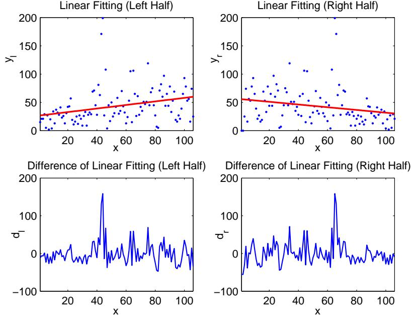
Figure 4.6: The process of how to calculate the PSNR from the central horizontal line of the DFT of a p-map. Take Fig. 4.5(d) as an example.
