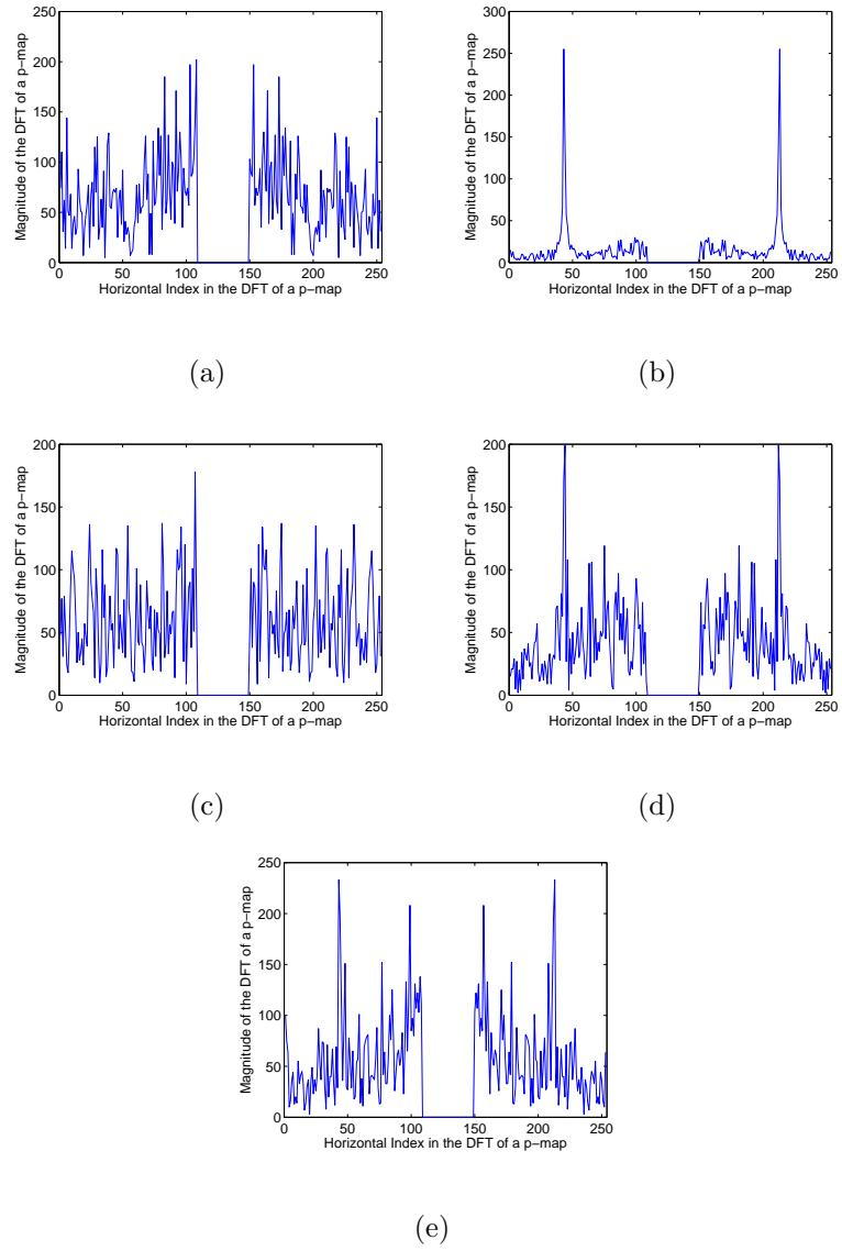
Figure 4.5: The central horizontal line of the DFT of the p-map of (a) an unaltered image, (b) a resized image, (c) a blurred image, (d) a blurred then resized image, and (e) a resized then blurred image.
