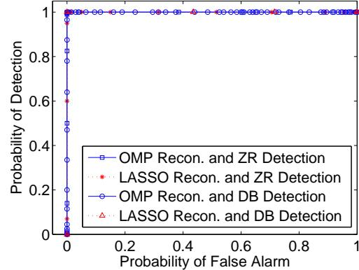
Figure 2.11: ROC curves of zero ratio detector and distribution-based detector on signals modeled as sparse signals in the presence of noise when different reconstruction algorithms were used.
