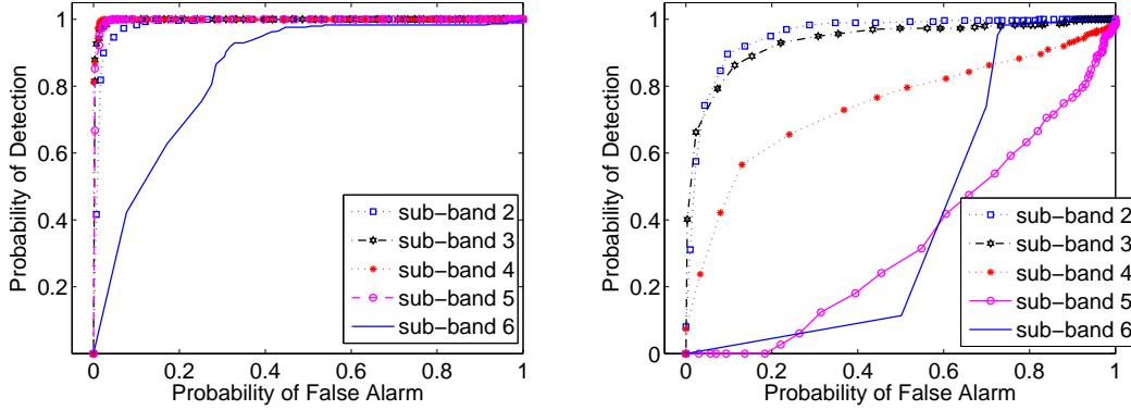
Figure 2.13: ROC curves of the first (left) and second (right) step detections on each DWT sub-band coefficients.  $M/N = 0.25$  is used in compressive sensing.
