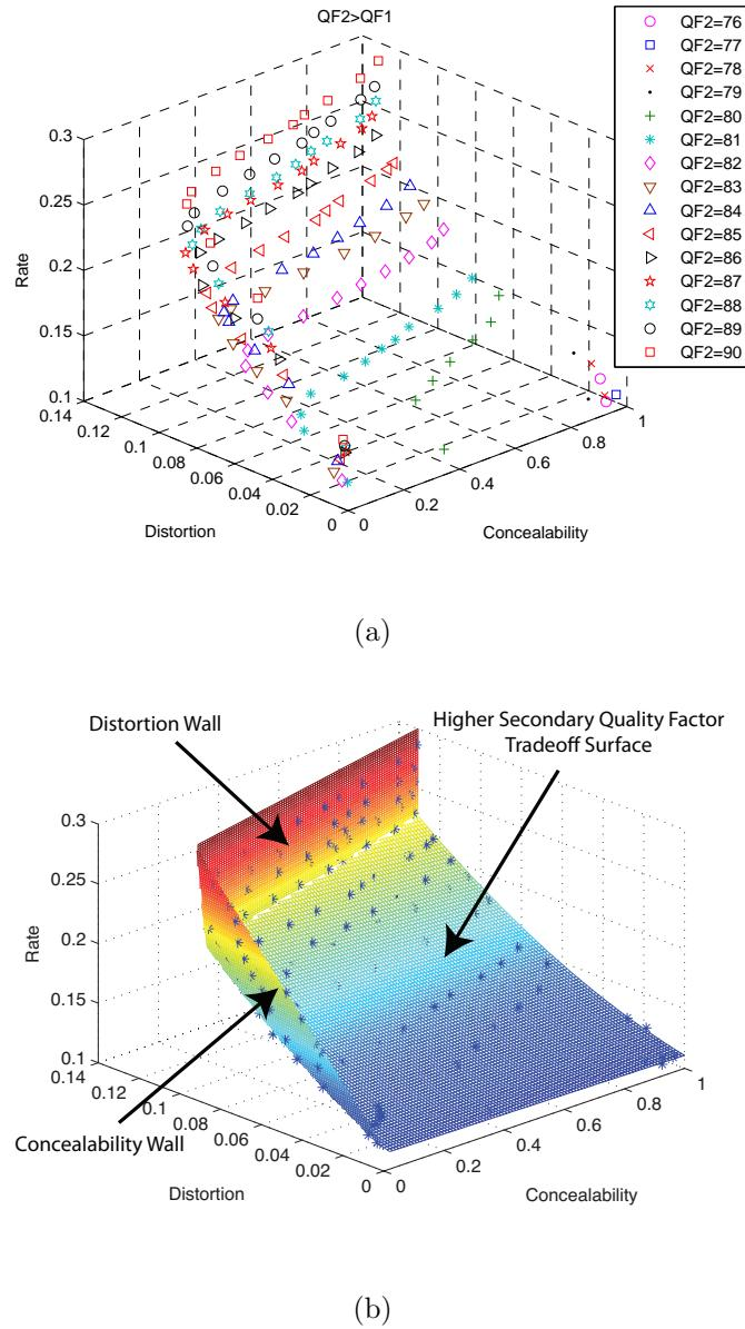
Figure 5.9: Tradeoff of concealability, rate, and distortion for the higher secondary quality factor case. (a) plots the R-D-C points. Points with the same marker and same color are those obtained by using the same secondary quality factor but different anti-forensic strengths. (b) is the polynomial fitting surfaces of (a).
