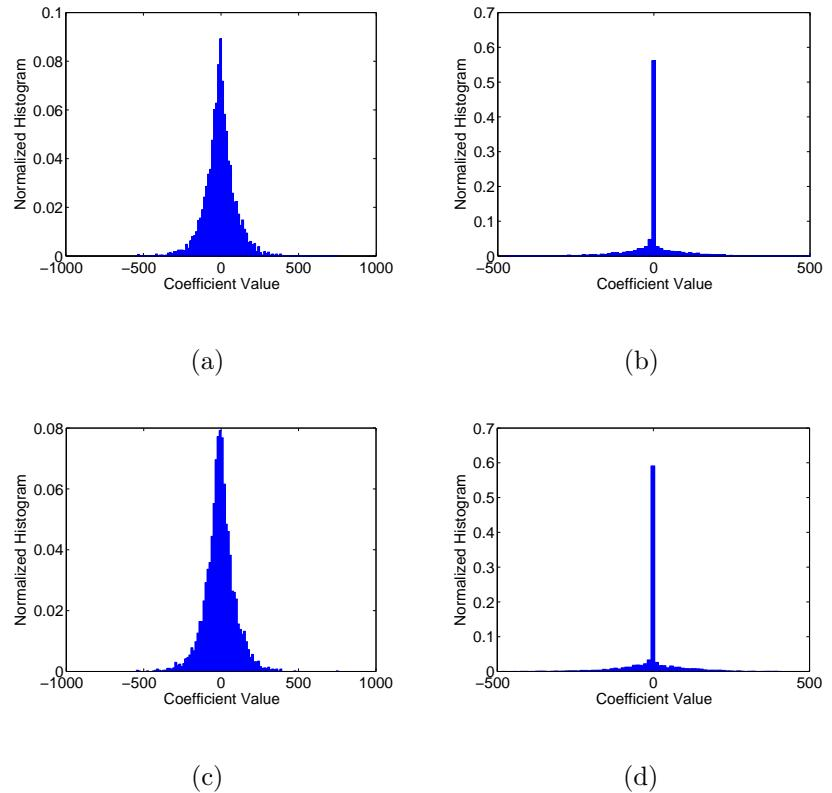
Figure 2.2: Example showing the fingerprints of compressive sensing in a nearly sparse signal with and without the presence of noise. The top row shows the histograms observed from a nearly sparse signal after (a) traditional sensing and (b) compressive sensing. The bottom row shows the histograms observed from a nearly sparse signal in the presence of noise after (c) traditional sensing and (d) compressive sensing.
