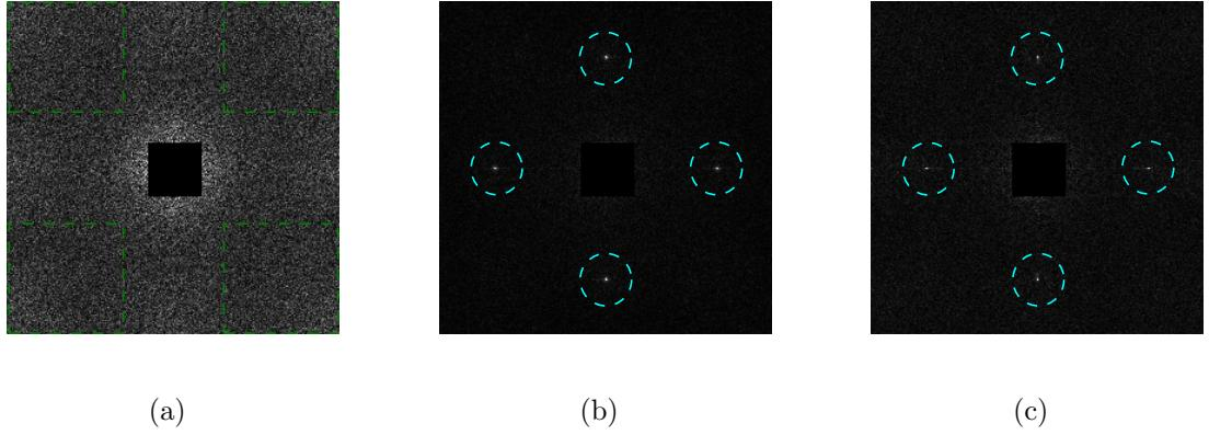
Figure 4.2: A confusing example that we may not be able to detect the order. Plotted are DFTs of the p-map of (a) the blurred image, (b) the blurred then resized image, and (c) the resized then blurred image when resizing factor is 1.5 and the variance of Gaussian blur is 0.7. Regions of interests are highlighted by dotted squares and circles.
