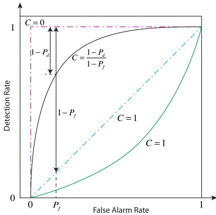
Figure 5.3: Examples of concealabilities related to ROC curves. When the detector achieves perfect detection, the forger has concealability of the fingerprints as 0. When the ROC curve is at or below the random decision line, we say that the forger has achieved concealability as 1. Then for those ROC curves between perfect detection and random decision, the concealability ranges from 0 to 1 and depends on a certain false alarm rate.
