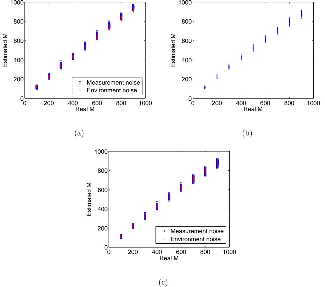
Figure 2.15: Estimated  $\hat{M}$  versus the real  $M$  for (a) sparse signals in the presence of noise, (b) nearly sparse signals, (c) nearly sparse signals in the presence of noise.
