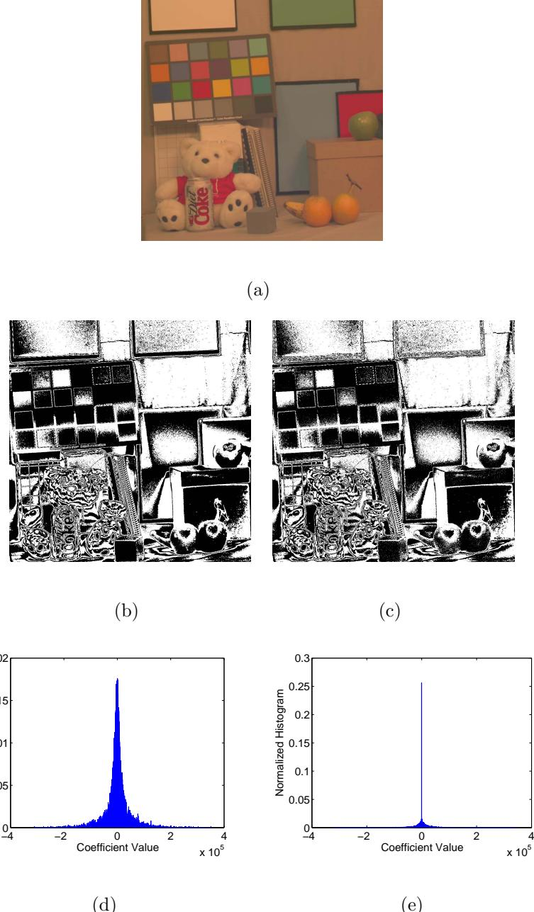
Figure 2.3: (a) A hyperspectral image taken from [9] with dimension  $1024 \times 1024$  pixel. (b) It's monochromatic image (obtained from raw data) corresponding to wavelength of 400nm. (c) The same monochromatic image obtained by compressive sensing and reconstructed from  $1024^2 \times 50\%$  compressive measurements. (d) and (e) Histograms of DWT subband 3 coefficients from (d) the traditionally sensed image and (e) the compressively sensed image.
