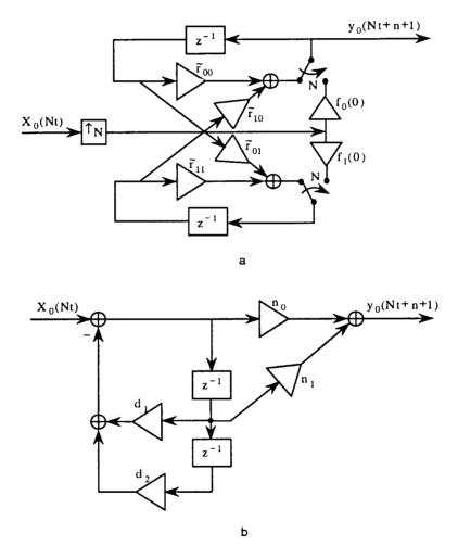
Figure 3.5: Inverse transform module.
