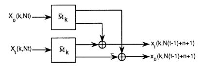
Figure 3.9: IDFT module for complex input.
