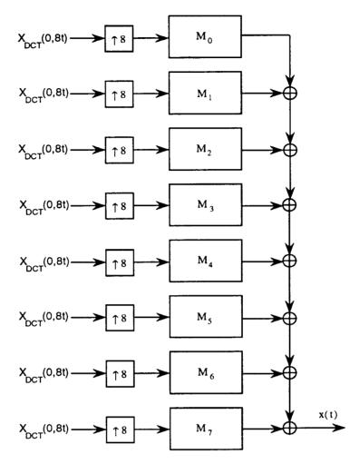
Figure 3.6: Recursive architecture for the IDCT.
