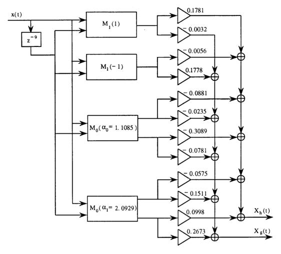
Figure 3.15: Architecture for the DWT filters specified in table 3.
