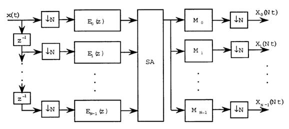
Figure 4.5: Decimated uniform-DFT bank using polyphase decomposition and time-recursive implementation for the IDFT.
