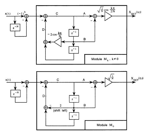
Figure 3.3: IIR architecture for the DCT kernel function.
