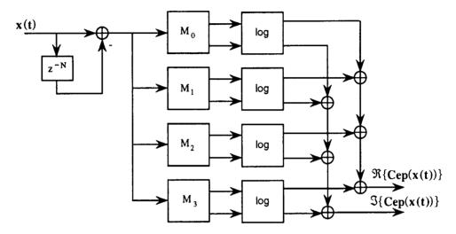
Figure 3.12: Cepstral transform architecture based on fast logarithm circuit.
