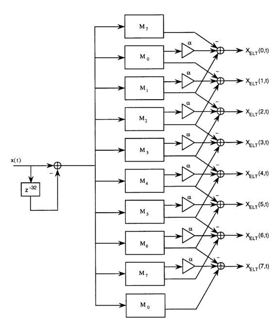
Figure 4.17: Time-recursive architecture for the ELT.
