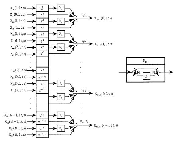
Figure 5.3: The Delay Add Array.
