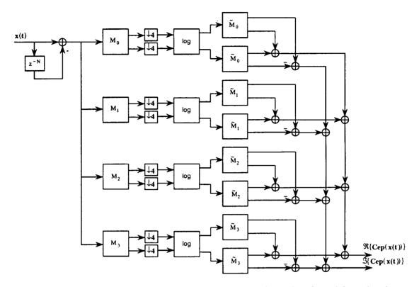
Figure 3.13: Cepstral transform architecture based on slow logarithm circuit.
