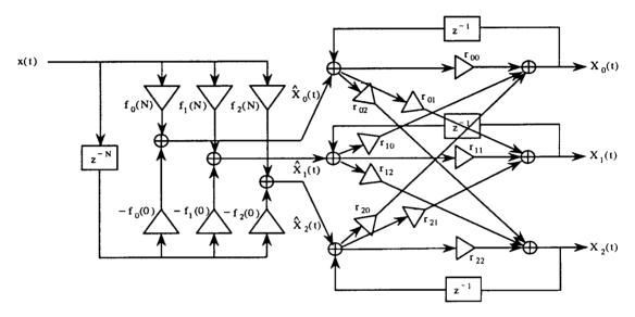
Figure 2.3: Lattice architecture for kernel group of size M=3.
