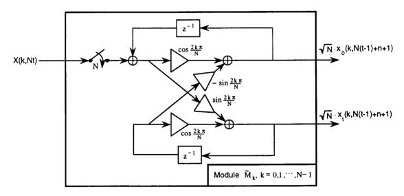
Figure 3.10: Details for real input IDFT module.
