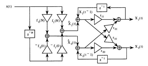
Figure 2.1: Lattice architecture for kernel group of size M = 2.
