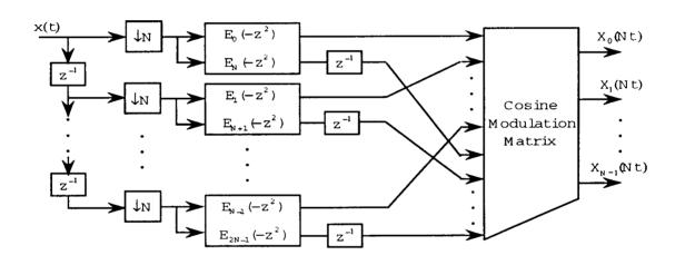
Figure 4.7: PR analysis bank based on cosine modulation.
