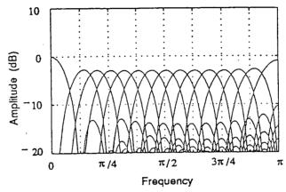
Figure 3.2: The magnitude responses of the DCT filter bank for N=16.
