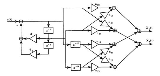
Figure 2.5: IIR architecture for M=2.
