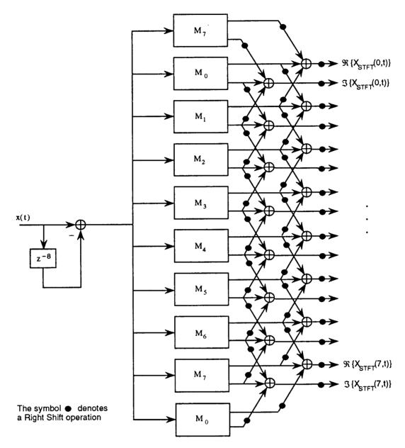
Figure 4.11: Time-recursive architecture of the STFT for N=8.
