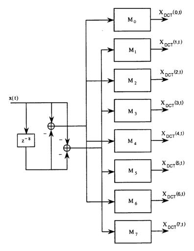
Figure 3.4: Recursive architecture for the DCT.
