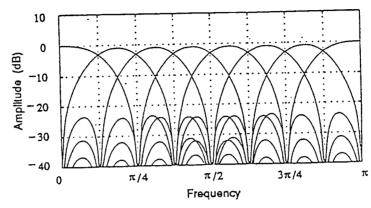
Figure 4.12: The magnitude responses of the MLT filter bank for N=8.
