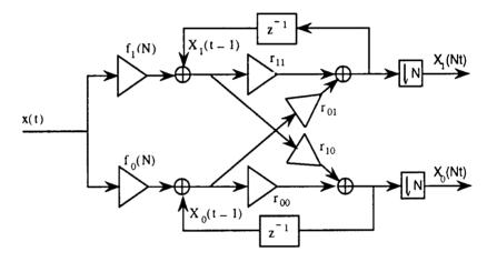
Figure 2.9: Lattice architecture for M=2 for an operator used in block transform.
