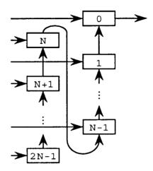
Figure 4.9: The Shift Array (SA) used in the PR QMF structure.
