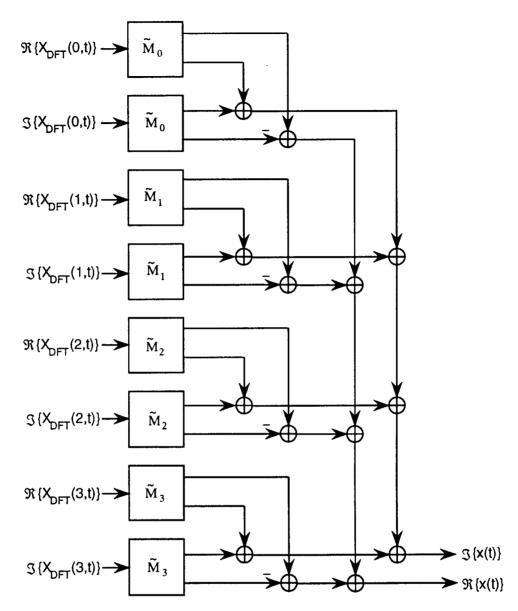
Figure 3.11: Recursive architecture for the IDFT.
