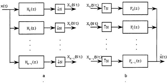
Figure 4.1: N-channel QMF bank: a. analysis system, b. synthesis system.
