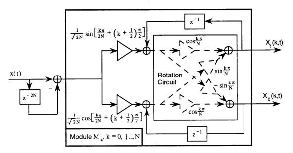
Figure 4.13: Lattice architecture for the MLT module.
