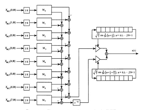
Figure 4.16: Time-recursive architecture for the IMLT.
