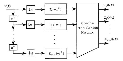
Figure 4.6: QMF analysis bank based on cosine modulation.
