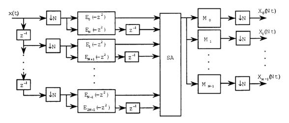
Figure 4.8: PR QMF analysis bank using time-recursive approach for implementing the cosine modulation matrix.
