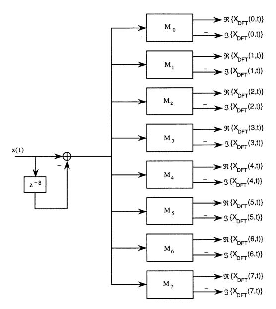
Figure 3.8: Recursive architecture for the DFT.
