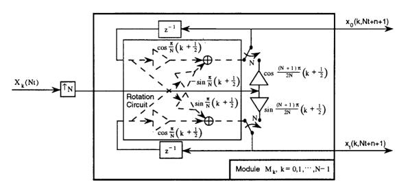
Figure 4.15: Lattice architecture for the IMLT module.
