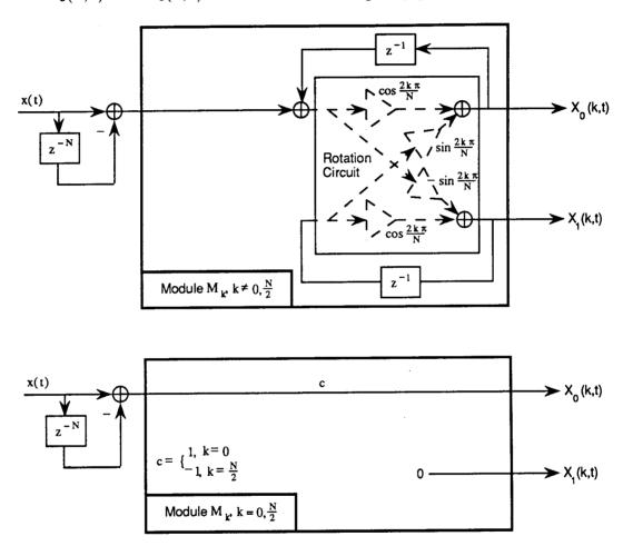
Figure 3.7: Lattice architecture for the DFT module.
