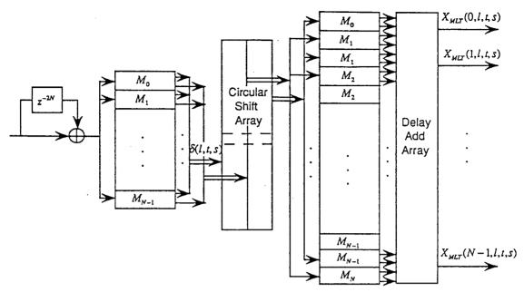
Figure 5.1: Recursive architecture for the 2-D MLT.
