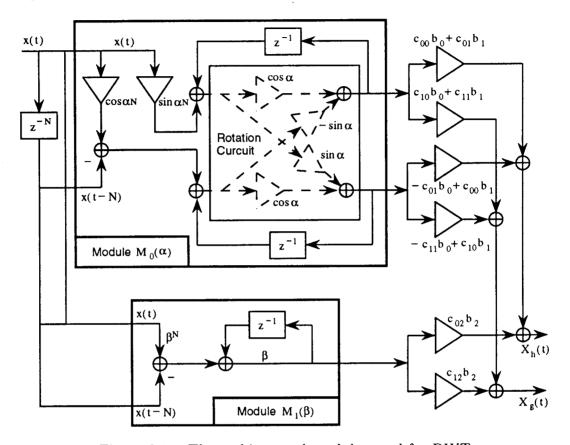
Figure 3.14: The architectural modules used for DWT.
