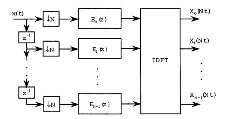
Figure 4.3: The uniform-DFT bank using polyphase decomposition.
