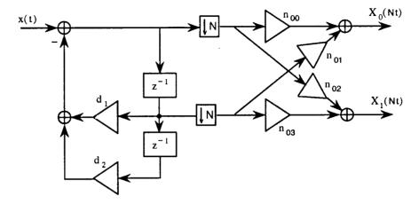
Figure 2.8: IIR architecture for M=2 for an operator used in block transform.
